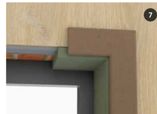
Door finish with MDF and door frame
