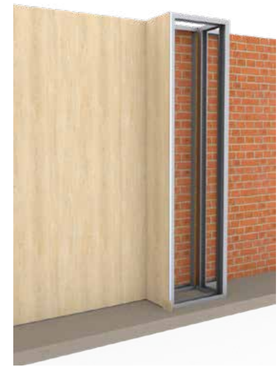
Method for positioning the aluminium profile in the external corner and U-construction:
