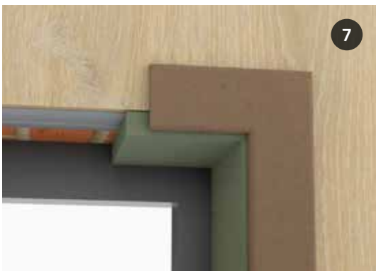
Door finish with MDF and door frame
